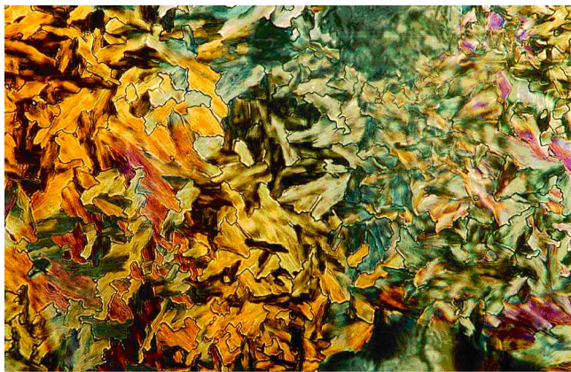
Figure 3. Optical texture of 2e at 120°C when viewed through crossed polarizing filters (200× magnification).
